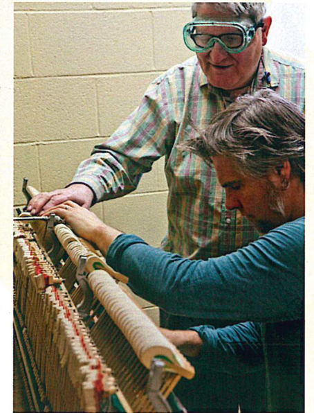
Don Mitchell, Director of Instruction, demonstrating how to check a piano regulation.
